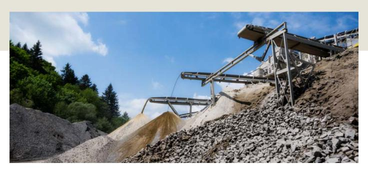
Conveybelts textile belting is designed from the inside out to withstand the heaviest of treatment when transporting materials such as coal, aggregates, timber and ore. The special inner fabrics compressed between layers of rubber have excellent adhesion and strength. The top and bottom covers are engineered to provide maximum protection of the carcass.
